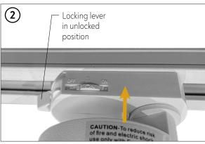
Ensure line voltage to the track is powered off. Insert the contact assembly into the track with the locking lever in the unlocked position.
